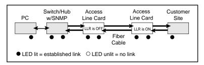
If one of the optical conductors is bad (as shown in the diagram box below), the card with LLR enabled will return a no link condition to its link partner. This aids the network administrator in determining the source of the loss.
